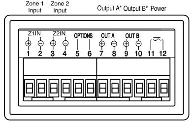
\* Output A is assigned to Zone 1 Input and Output B is assigned to Zone 2 Input. If necessary, the input/output relationships may be reversed. See 5P to in Secure Menu.
